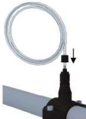
Thread the PE tubing through the cap and push it onto the valve cone.
