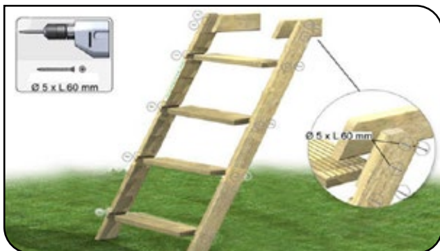
Figure 61 – Assemble the wooden ladder
