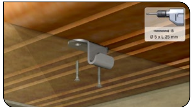
Figure 62 – Hook beneath the coping
