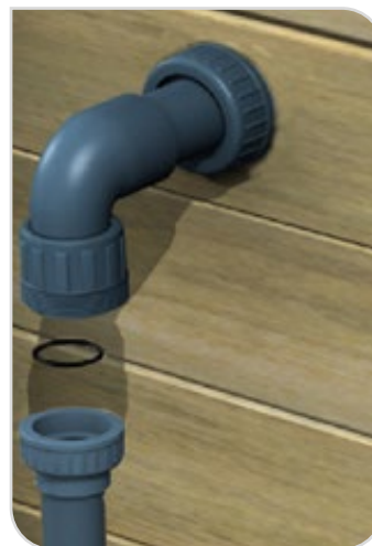
Figure 44 – Rigid descending pipe under the return fitting (Odyssea model)
